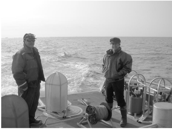
FIG. 5. DASAR on deck with anchor and tag line, ready for deployment. Also on deck are other DASARs without their protective socks.
